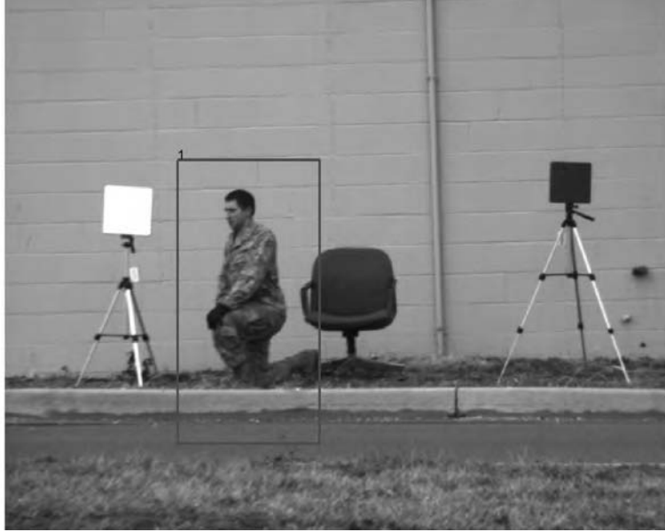
Figure 1. An example of the results from the skin-cued dismount detection system with a bounding box placed around the detected dismount.
