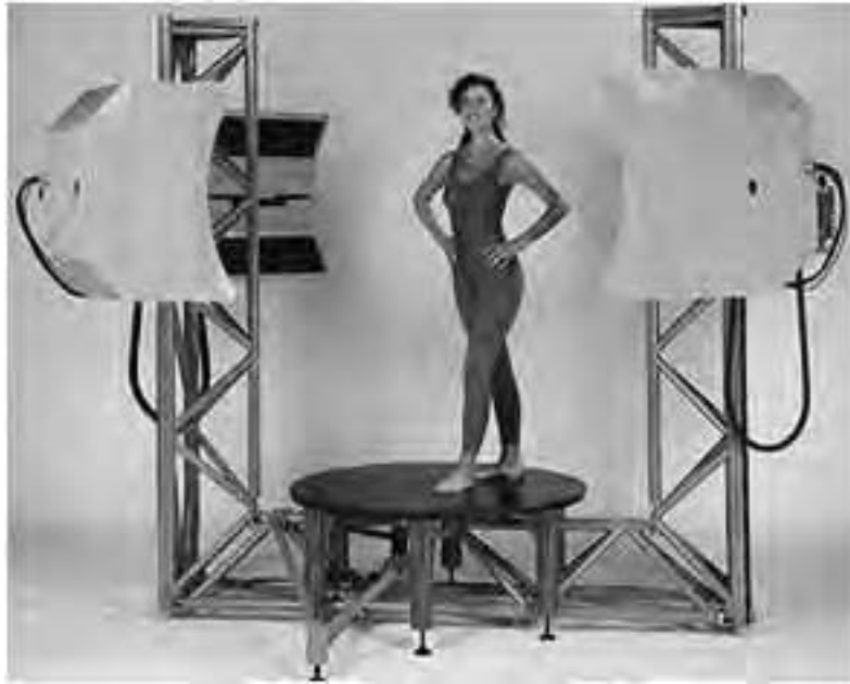
Figure 44. The type of scanner used to obtain 3-D body scans in the CAESAR database.
